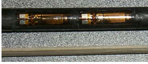
Figure 3: These two uniaxial strain gauges (EK-06-250BF-10C) each have nominal resistances of approximately 1000\Omega and are 6.35mm long and 3.18mm wide each.
