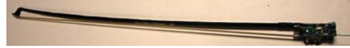
Figure 5: The Hyperbow consists of a modified Cod-aBow Conservatory violin bow enhanced with strain sensors and a resistive strip used for position sensing. A PCB mounted to the frog houses the accelerometer sensors as well as control circuitry for sending data wirelessly to a remote receiver.
