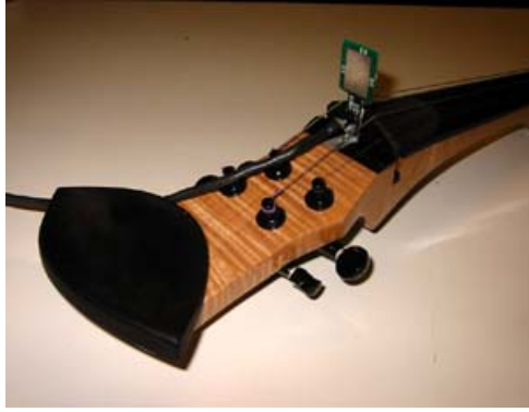
Figure 1: The electrode antenna is mounted behind the bridge of a Jensen electric violin.
