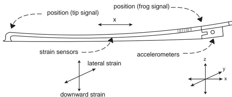
Figure 3.17: The third and final prototype of the *Hyperbow* included accelerometers, mounted at the frog of the bow, to give acceleration data for all three axes of bow movement, two strain sensors, mounted around the middle of the stick, for downward (normal to the strings) and lateral (parallel to the strings) strains, and the outputs for the two signals necessary for position sensing (parallel to the bridge), located on the stick at the extreme ends of the bow hair.
