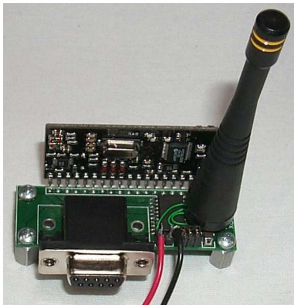
Figure 3.2: The printed circuit board designed to receive the accelerometer and strain data from the *Hyperbow* was very simple, containing only the Linx 1/4 wave whip antenna (ANT-916-CW-QW), the Linx RXM-900-HP-II receiver, a MAX233 RS-232 level converter, and a serial port. (Note: The three green wires depicted here were included to correct an error in the implementation of the MAX233 chip.)
