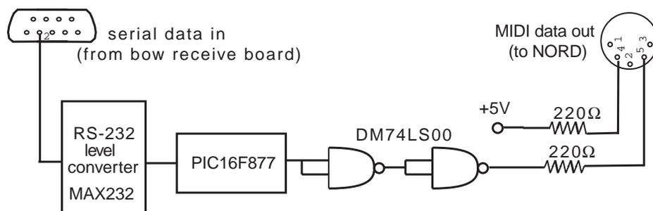
Figure 5.2: The serial to MIDI converter used in the Nord Modular demo setup was constructed with a MAX232 RS-232 level converter (to bring the serial signal down to the 0-5V range); a PIC16F877 microprocessor that read the serial data, truncated it to the 7-bit MIDI range, and sent it out in MIDI format; and a DM74LS00 NAND gate chip used to buffer the signal before sending it through the MIDI port.
