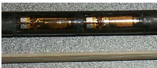
Figure 3: These two uniaxial strain gauges (EK-06-250BF-10C) each have nominal resistances of approximately 1000\Omega and are 6.35mm long and 3.18mm wide each. The winding of the metal alloy wire that composes the gauge can be seen running back and forth in the direction parallel to the bow. The terminals of this wire are connected to solder tabs.
