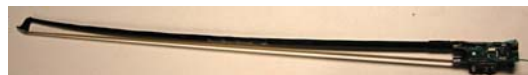
Figure 5: The Hyperbow consists of a modified CodaBow Conservatory violin bow. This bow was enhanced with strain sensors and a resistive strip used for position sensing. A PCB mounted to the frog houses the accelerometer sensors as well as control circuitry for sending data wirelessly to a remote receiver (see text).
