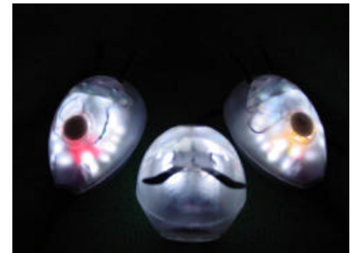
Figure 51. Clusters of color LEDs in the final version of the Beatbugs. Flushing white LED signifies the rhythmic motif. Red and yellow LED clusters signify bending the left and right antenna respectively.
