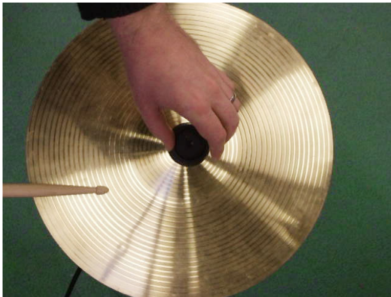
Figure 6-4: Cymbal pitch controlled with knob
