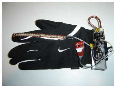
Illustration 27: Gesture Glove with sensors and Funnel I/O board
