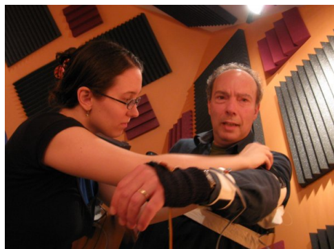
Figure 16. The author fits Disembodied Performance sensors on James Maddalena Accelerometers on the hands and forearms measure qualities of Maddalena's movement. Photo by Tod Machover.
