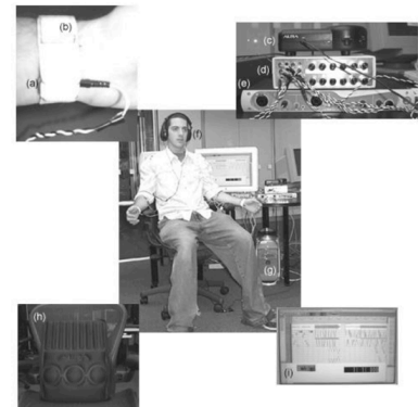
Figure 8: Photograph of Skinscape system. (a) V1220 transducer located on wrist; (b) Velcro adjustable elastic band; (c) Interactor cushion amplifier unit; (d) 12-channel V1220 amplifier unit; (e) Digi001 hardware interface; (f) ATX-M3H headphones; (g) Macintosh G4; (h) screenshot of ProTools LE audio editing environment. (From (Gunther, 2001))
