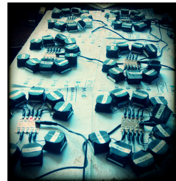
Figure 3.59. Charging batteries for Bluetooth audio receivers to create a Bluetooth Location Network in the performance space.
