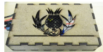
Figure 3.53. The final design of a wearable computing system. The on-site participants carried this box in a fanny pack which was then connected to the sensors and actuators in the mask.
