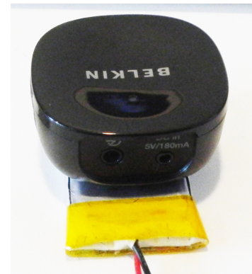
Figure 3.58. A Bluetooth audio receiver that was used as the location tracking device.
