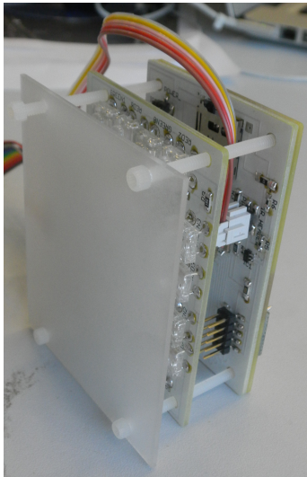
Figure 3.12. The final circuit board design. A diffuser is on the top layer followed by the LED board, the main controller board, and the radio board.
