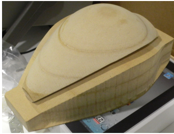
Figure 3.11. An MDF mold for thermoforming HDPE.
