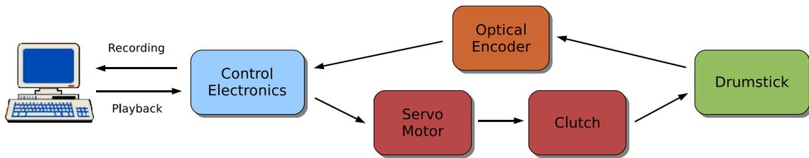
Figure 3-4: Functional diagram of the Haptic Guidance System (HAGUS)
