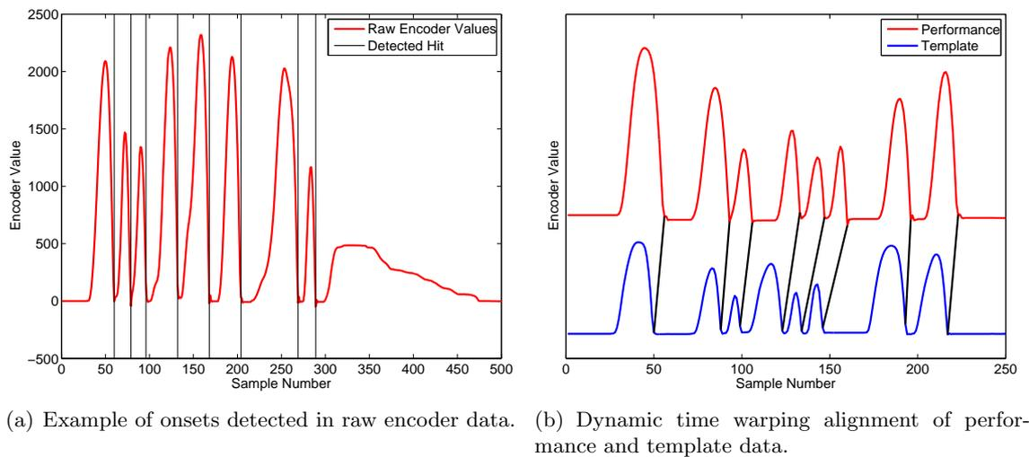
Figure 4-2: Onset detection and alignment of subject data.
