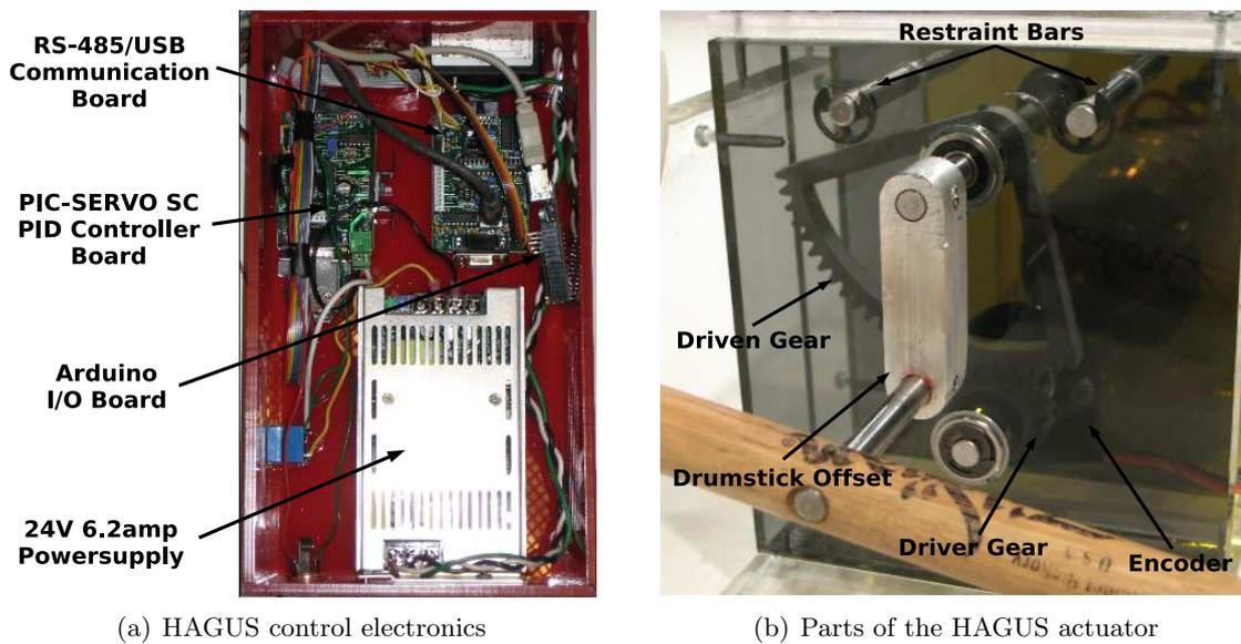
Figure 3-6: Electronic and hardware components of HAGUS
