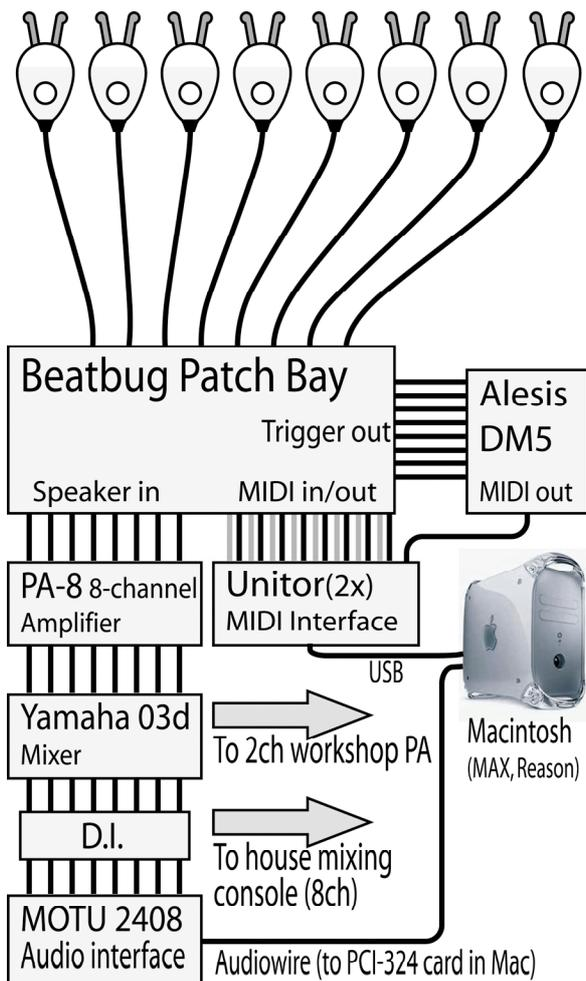
Figure 2. Beatbug rack schematic.
