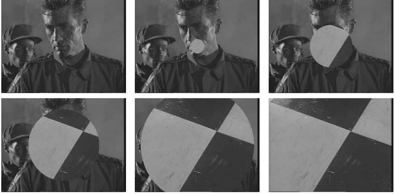
Figure 6-2. Using a time-varying alpha-blending matrix to transition between two video sequences.
