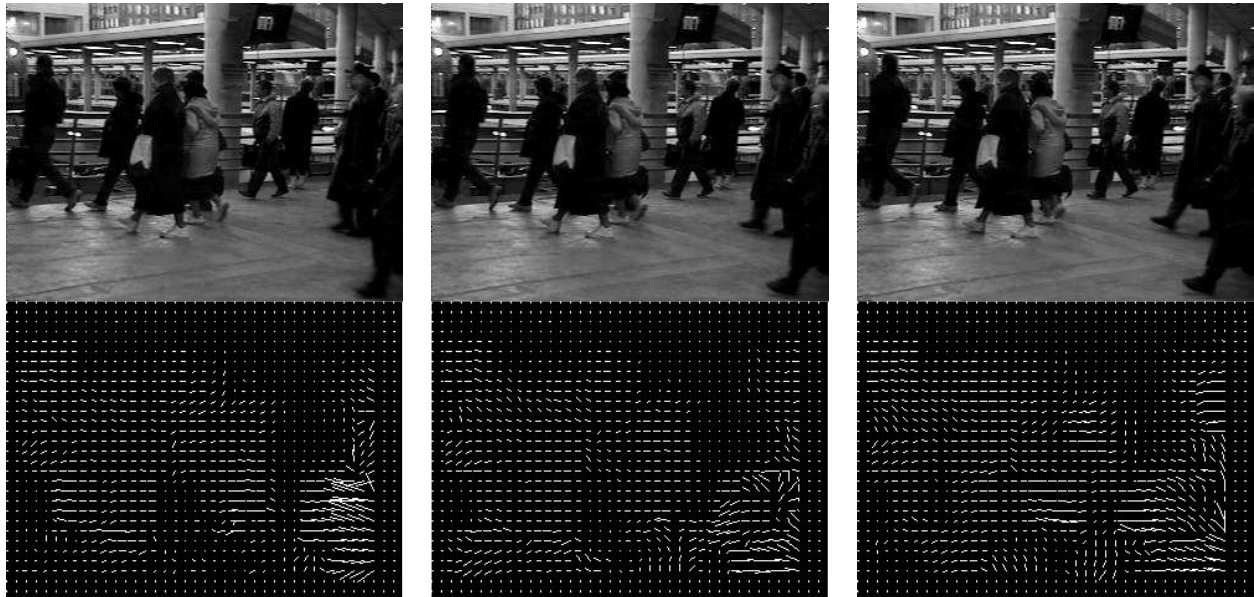
Figure 4-3. Three frames from a video sequence and their corresponding optical flow.
