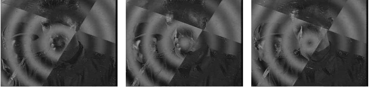
Figure 6-3. Using a radial "wave" as the source to an alpha-blending algorithm. The center of the screen is the origin of the effect, radiating outwards over time.
