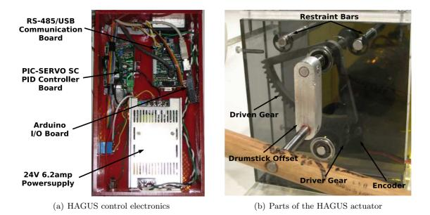
Figure 3-6: Electronic and hardware components of HAGUS
