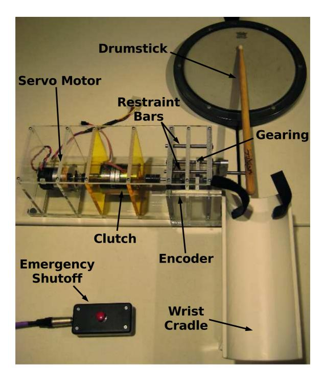
Figure 3-7: The Haptic Guidance System hardware
