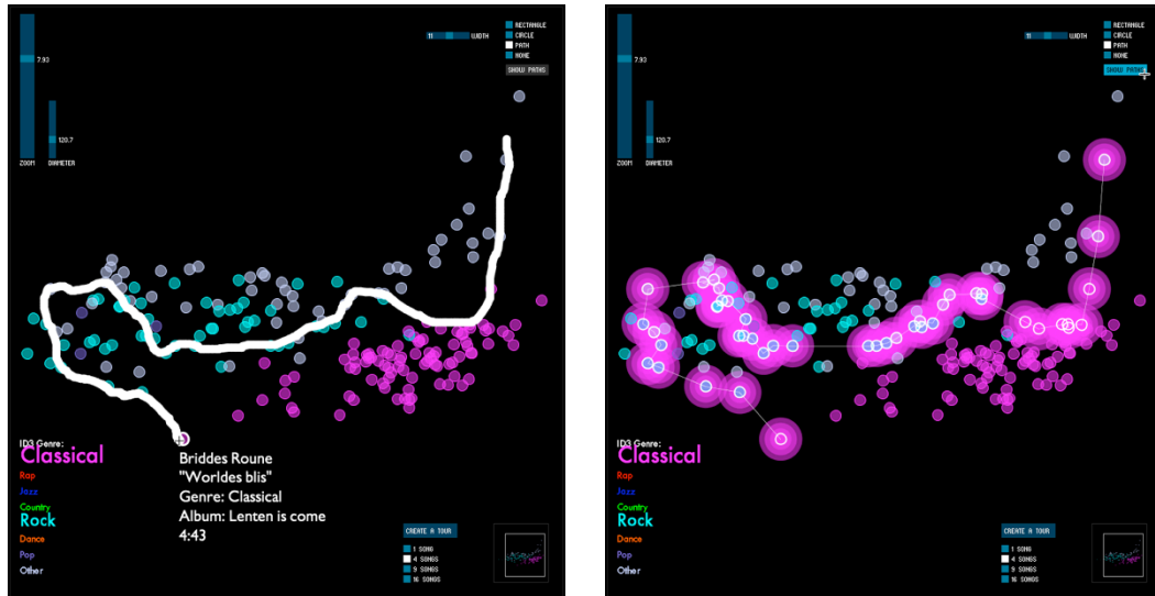
Figure 5-5: Path selection tool, as the user defines the selection (left) and the resulting selection (right). The user can select songs along a path through the space.
