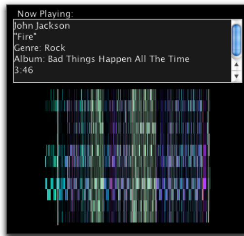
Figure 5-16: Song information. Metadata and soundsieve image for the current (or most recent) song are displayed. A white vertical line moves across the soundsieve image during playback, indicating the current location in the song.
