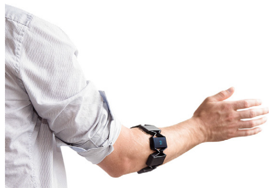
Fig. 34 MYO armband placed on forearm
