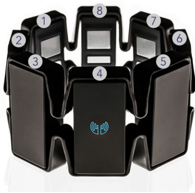
Fig. 33 MYO armband with numbered EMG-sensors
