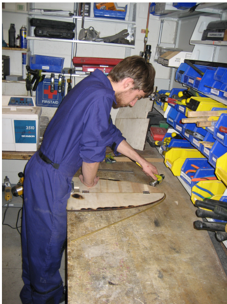
Figure 4.24 The manual formation of the curved brass frame using a laser-cut plywood template.
