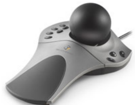
Figure 4.37 3D Connexion Spaceball used for the spherical control interface to the Chandelier.
